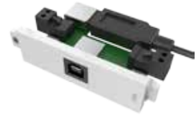
TC3 USBB+ [SAP:3446582] USB-b module with active booster circuit. USB 2.0 Maximum input cable length: 10m. Note: Uses 5v from USB. For longer cables external power may be required.
