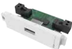
TC3 USBPW [SAP: 3985223] Active USB charging module. Auto current adjustment. Comes with 12 volt / 2 amp power supply. Power through so it can share a PSU with other 12v Vision products.
