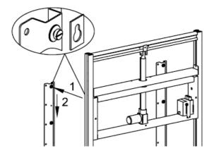
3. FIT BRACKETS to side of frame as shown. Add locking screws to prevent frame being lifted off legs.
