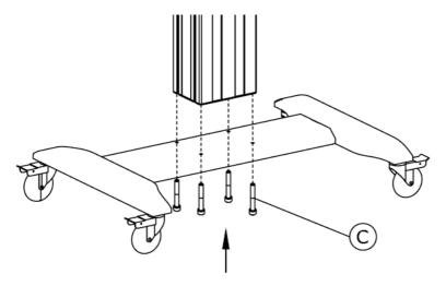
4. FIX FLAT-PANEL BRACKETS TO REAR Common M6 and M8 bolts are included. See the flatpanel manual to check which bolts to use.
