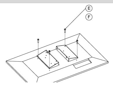
5. HANG FLAT-PANEL ASSEMBLY ON COLUMN Once in place fit locking screws (step 2).
