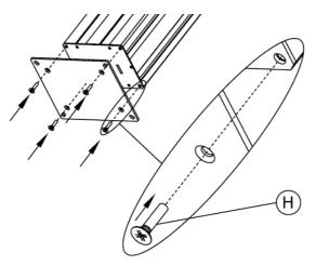
b. FIX COLUMN ASSEMBLY TO WALL
