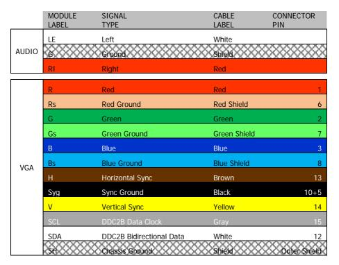
Note: There is no colour standard for the Horizontal and Vertical Sync cables, so if you use cables not included with the Techconnect, you will need to use a continuity tester to determine which colour on your cable matches which pin on your cable.
