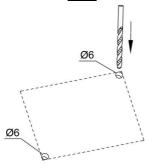
3. CUT HOLE Use a jigsaw. As the bezel on the TC2-TILT2 is very thin this must be cut accurately.
