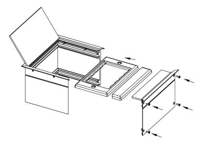
5. OPTIONAL: ADJUST CHASSIS DEPTH It may be necessary to make the chassis shallower. A cutting slot is moulded into the product to use as a guide.
