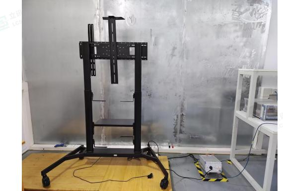
Photo of Power Line Conducted Measurement
