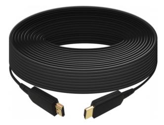
Long HDMI cable which is thin and flexible. Uses Multimode optical fibre wrapped in synthetic Aramid fibres which are heat-resistant and strong synthetic fibres used for ballistic-rated body armour fabric.
