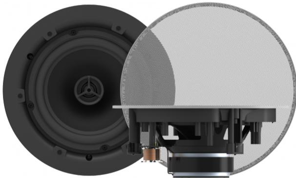
The CS-1800 ceiling speakers feature a two-way design. They use the ceiling void as an infinite baffle – allowing un-damped driver excursion – all of which adds up to rich, detailed sound. The main driver is a 6.5" polypropylene cone complimented by an advanced 0.5" tweeter. These low impedance speakers do not sacrifice frequency range like 100/70v line speakers do. Perfect for meeting spaces.
